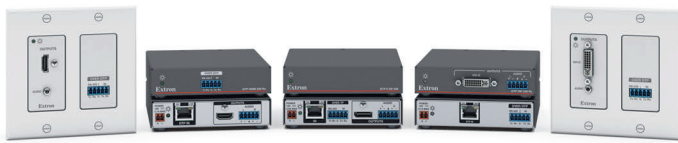
Figure 16: DTP receivers provide convenient connection points at remote display locations, extending video, audio, and control signals up to 330 feet (100 meters) over a shielded twisted pair cable from a DTP receiver or other DTP-enabled product.
