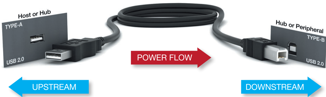
Figure 7: USB 2.0 cable showing connection types and power flow
